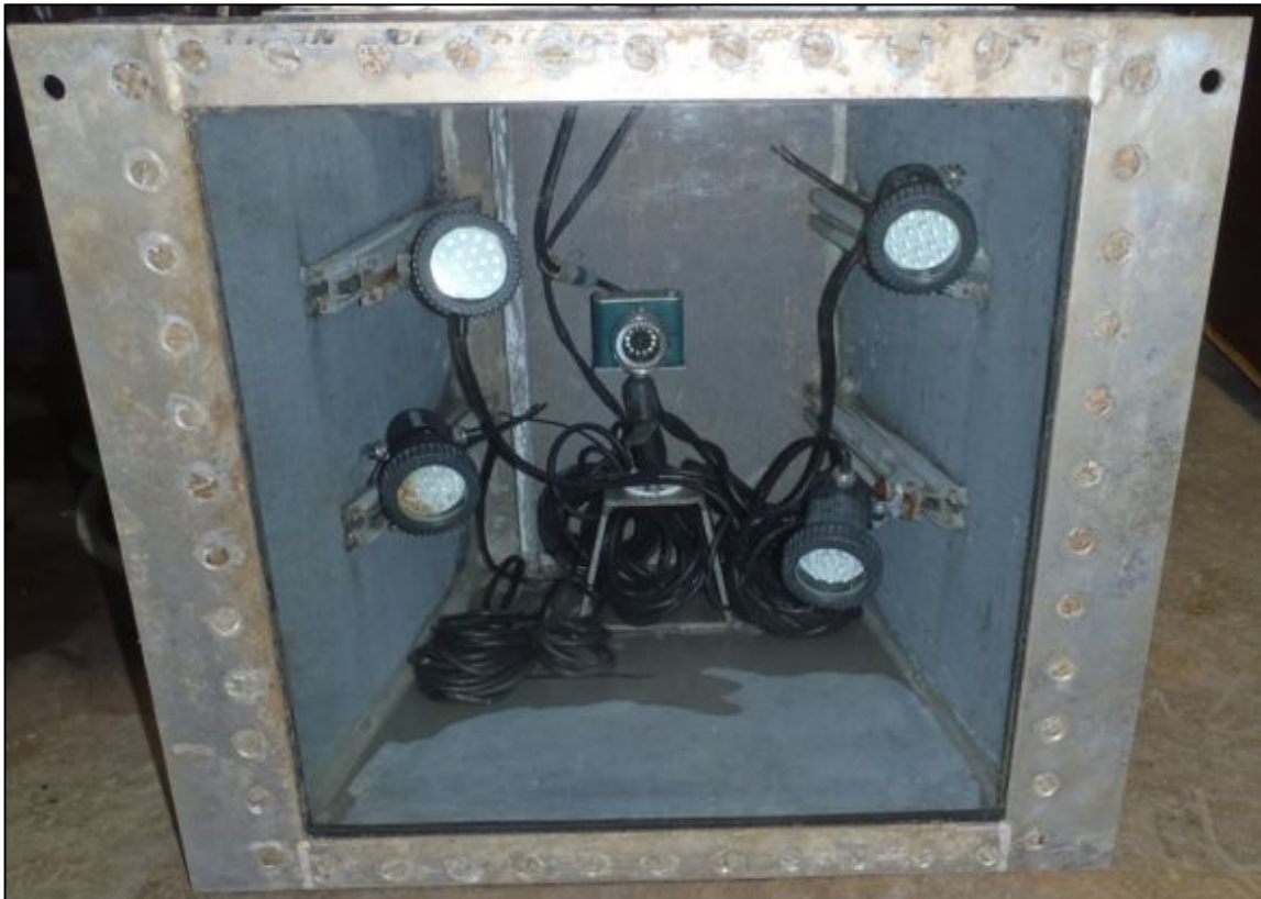
Figure 3.10: Underwater video camera installed on the Milwaukee River fishway, Wisconsin, by the US Fish and Wildlife Service for the Ozaukee County Planning and Parks Department.
