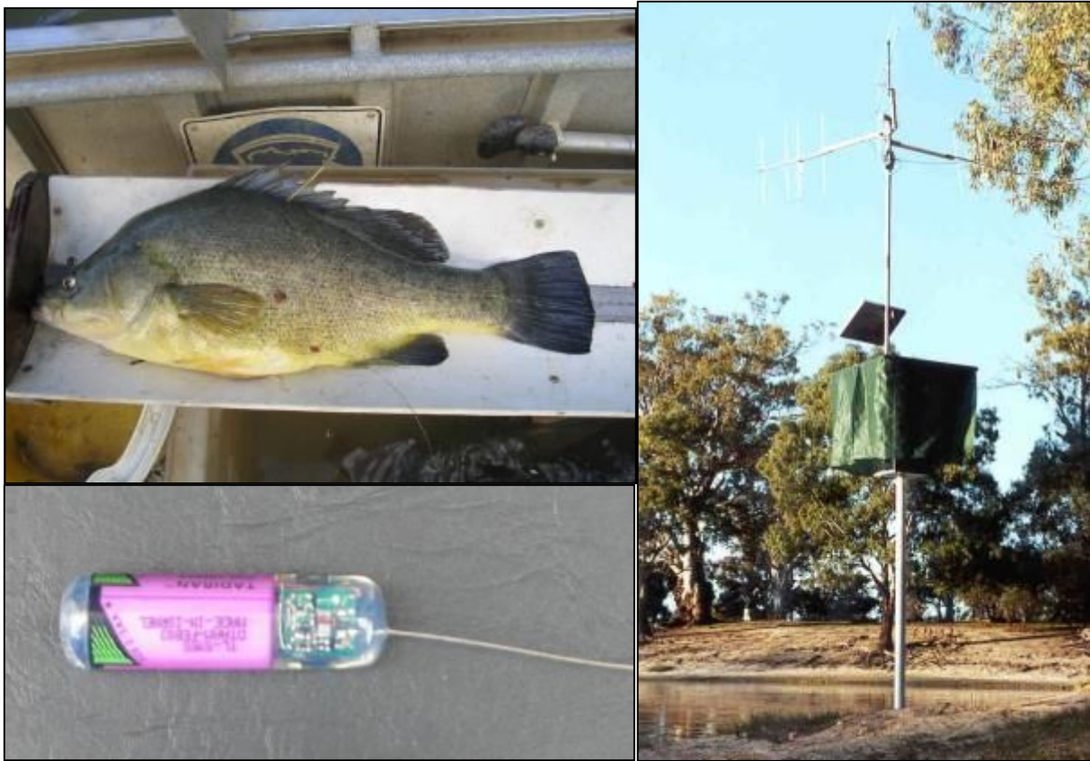
Figure 3.8: Top left: Golden perch with external dart tag and radio-transmitter implanted. Bottom left: Radio tag. Right: Radio-tracking tower with directional antennas at the junction of a river anabranch to track the movements of fish.
