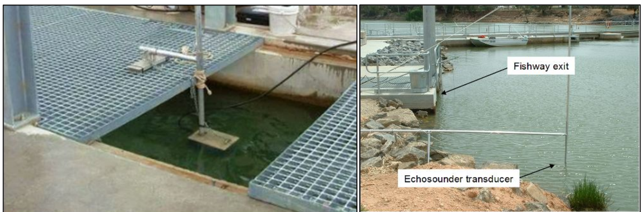
Figure 3.11: DIDSON sonar installed on a fishway exit (left), and split-beam hydroacoustics unit installed on the exit of a fishway (right).
