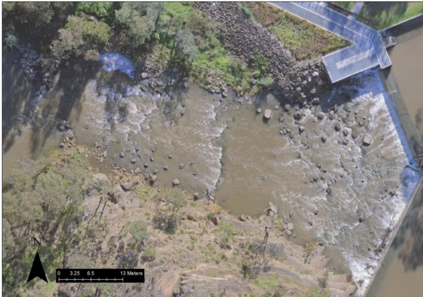
Figure 5.1: Digital elevation map of the rock-ramp fishway downstream of Dights Falls weir.
