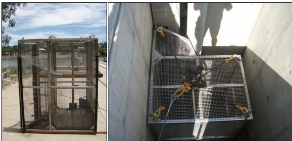
Figure 3.1: Fishway trap used to sample vertical-slot fishway (exit), and in position (entrance).
