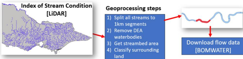
Figure 1. Overview of the waterbody (A) and river/stream (B) GIS layers and processing steps used to derive estimates of the number of waterbodies, rivers and streams with surface water in Victoria.
