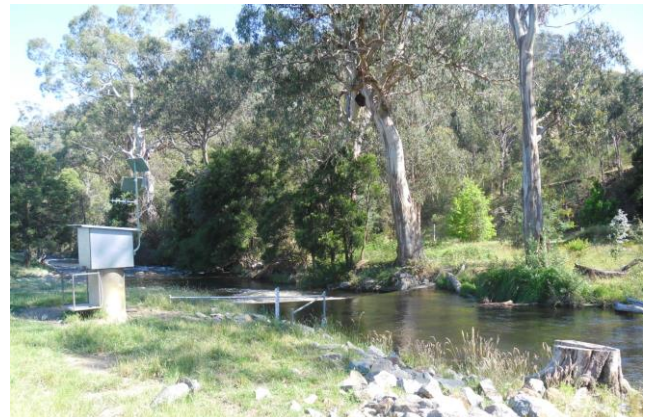
Figure 1: A typical stream gauging station (Photo: DELWP)
