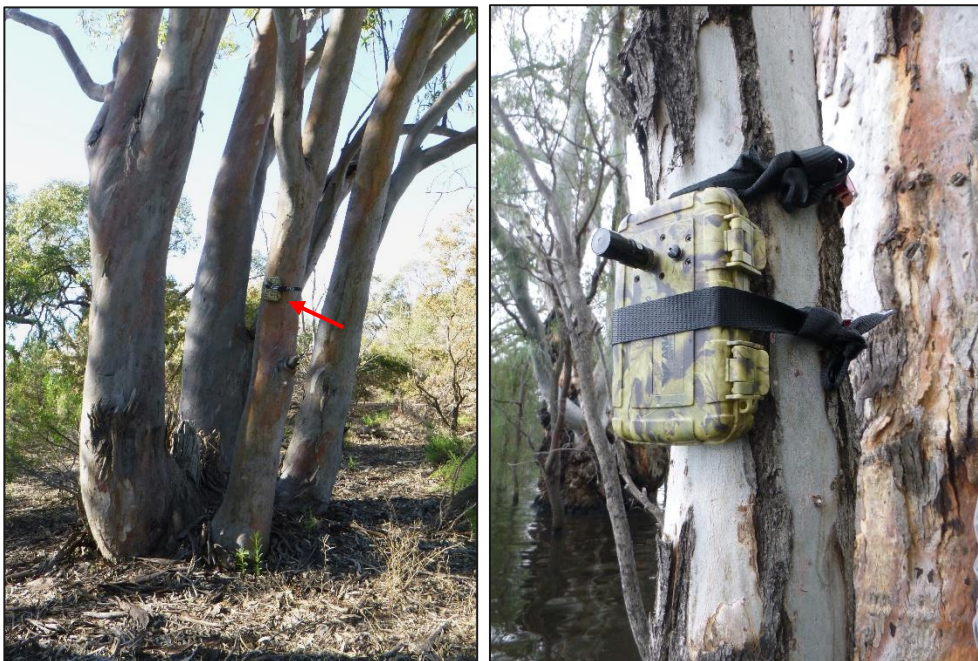
Figure 3. Anabat Swift detector with omnidirectional microphone, set approximately 1.5 m above the ground, pointing towards the lake.
