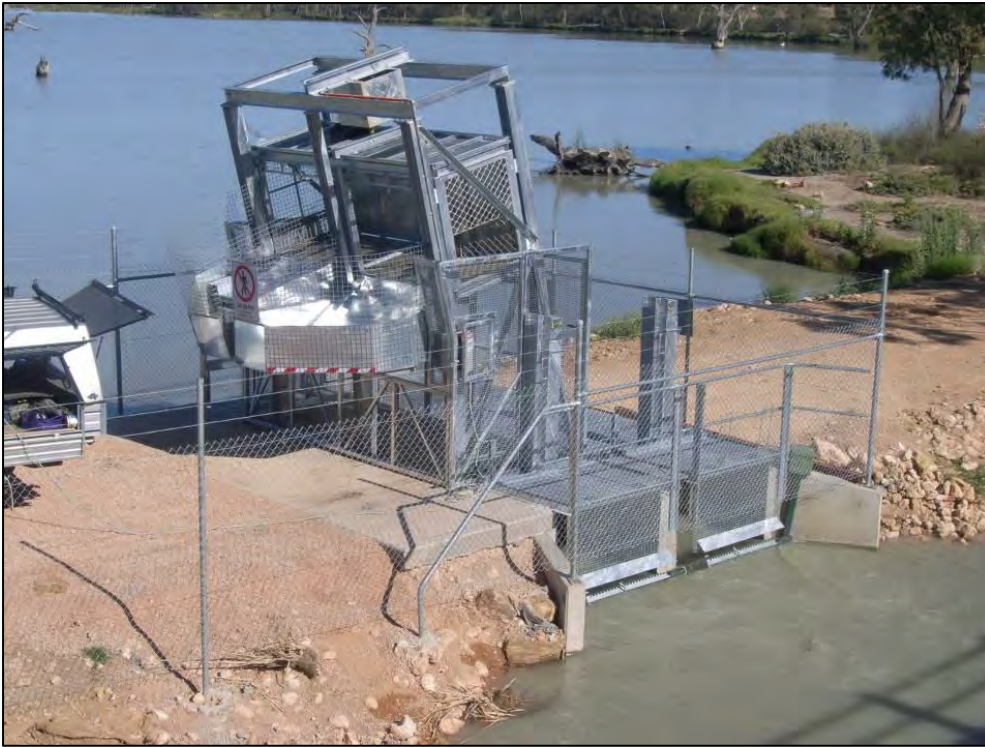
Figure 8. Photograph of the Wetland Carp Harvesting System at Lake Bonney, incorporating the Williams' Carp separation cage, gantry, hoist, Carp pivot screens and Carp deflector screens (Thwaites 2011)
