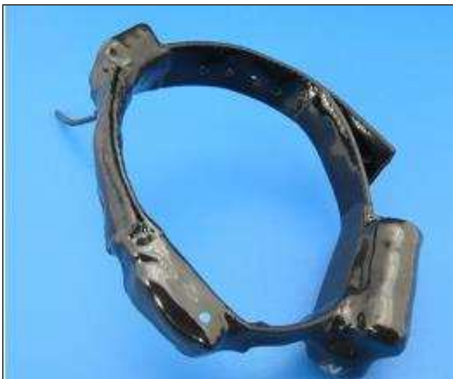
Figure 4. Telenax GPS collar for foxes at Hattah–Kulkyne National Park.
