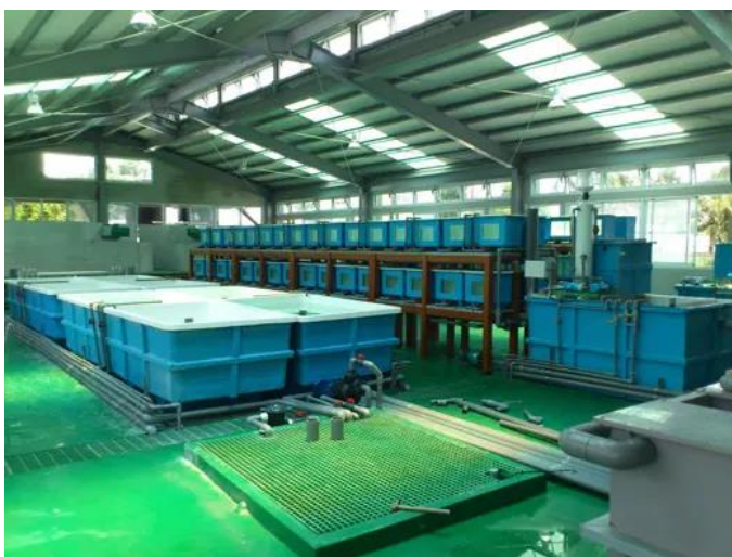
Figure A3-3. Example of recirculation system (Taiwantrade.com)
