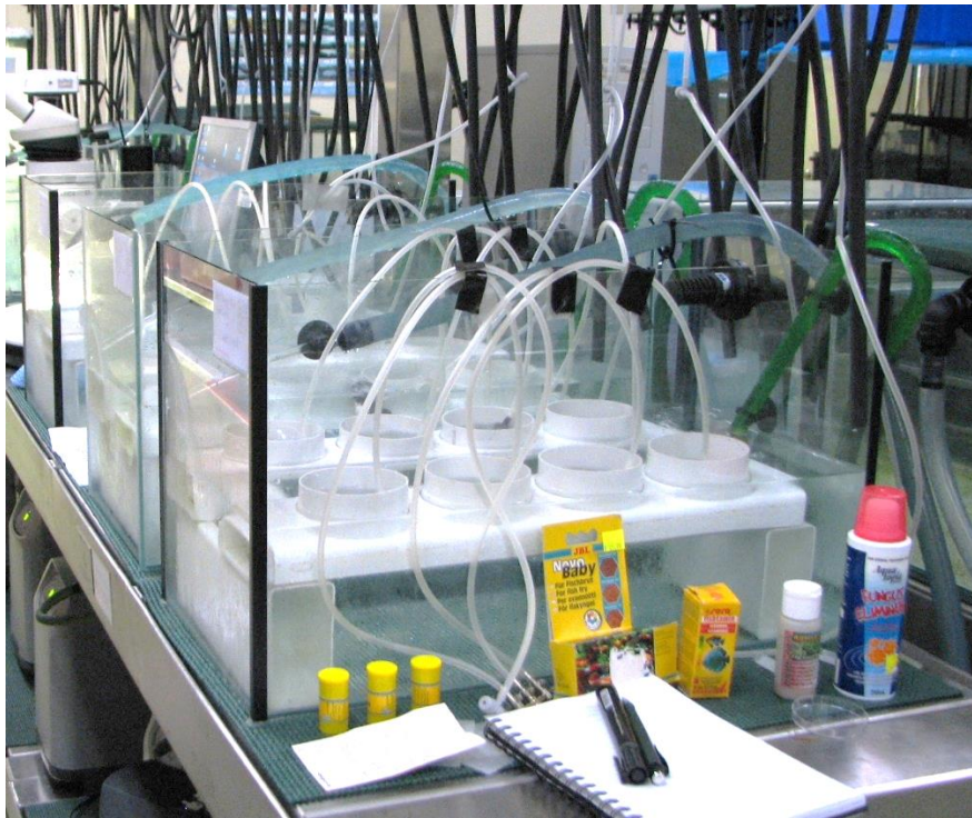
Figure A1-4. Circular egg incubators in a 20L glass aquarium (Imaged: Dan Stoessel)
