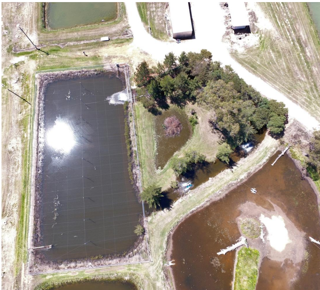
Figure 3. Netted 0.18 ha earthen pond and associated artificial stream used to maintain broodfish at the Narrandera Fisheries Centre (image: NSW DPI).
