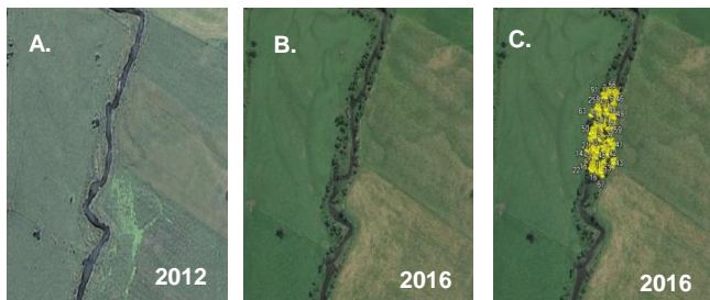
Figure 1. Aerial images (A)(B) of the same site over time are used to measure rates of change in the cover of woody vegetation after management by assigning a vegetation cover type to 100s of georeferenced points (yellow points in C.).
