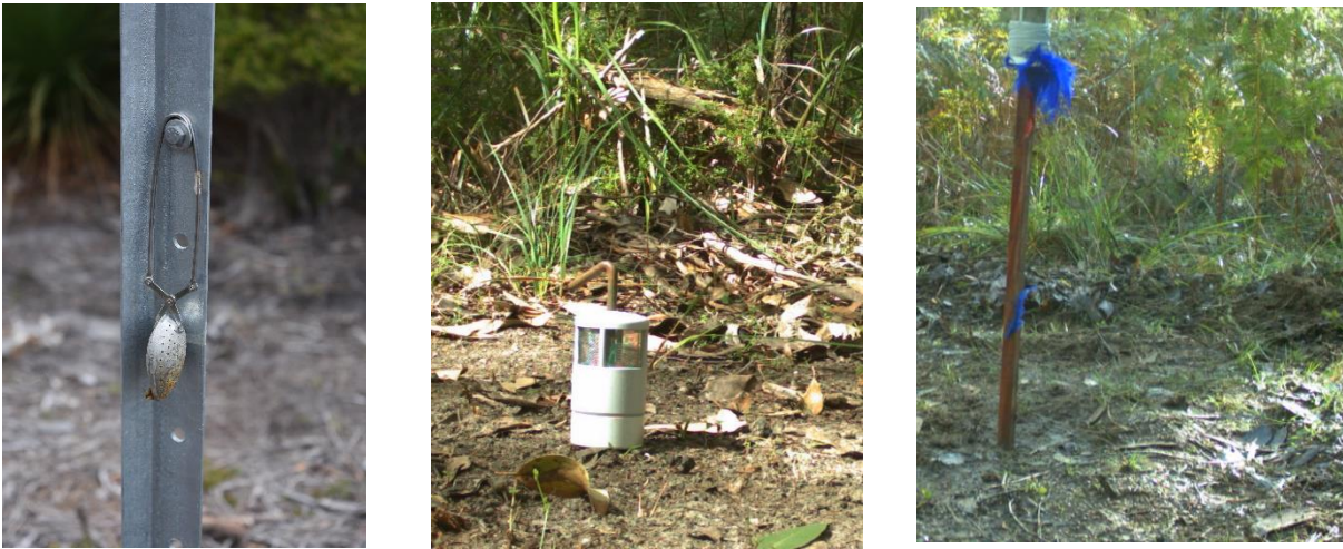
Figure 2. Lure holders used in camera traps were either a tea infuser or vented cowling.
