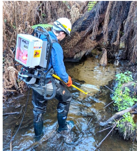
Fig 3. Backpack electrofishing in the upper Timbarra River (Photo credit: Michael Nicol DELWP)
