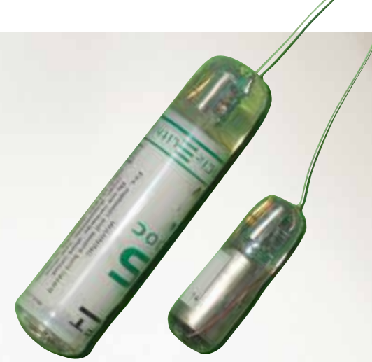
Radio transmitters which are surgically implanted into fish
