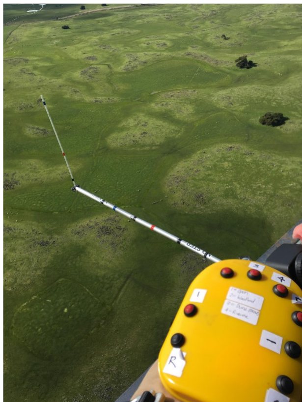
Figure 4. Sighting poles are used to place detected animals into distance categories from the aircraft (photo credit – Mark Lethbridge, EcoKnowledge).
