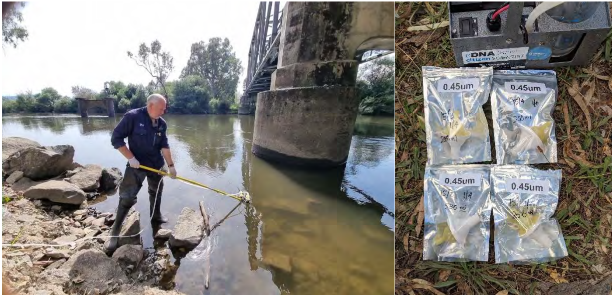
Figure 3. eDNA water sampling (left) and pump and filters (right). Image credits: Daniel J. Stoessel (left), Tarmo A. Raadik (right).
